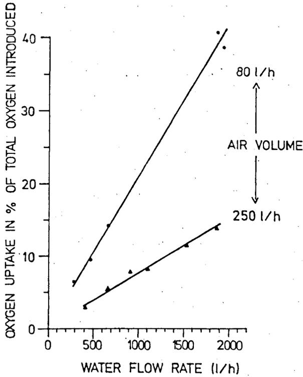
Fig. 5: Oxygen transfer rates in relation to water flow rate and air supply
