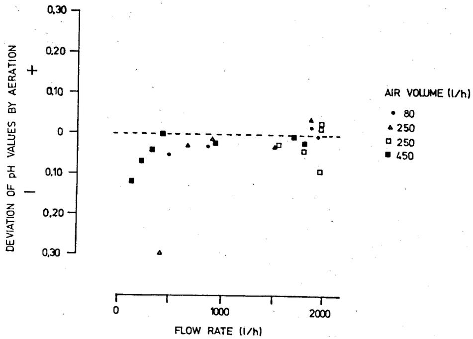
Fig. 7: Changes in pH values in relation to air and water flow rates.
