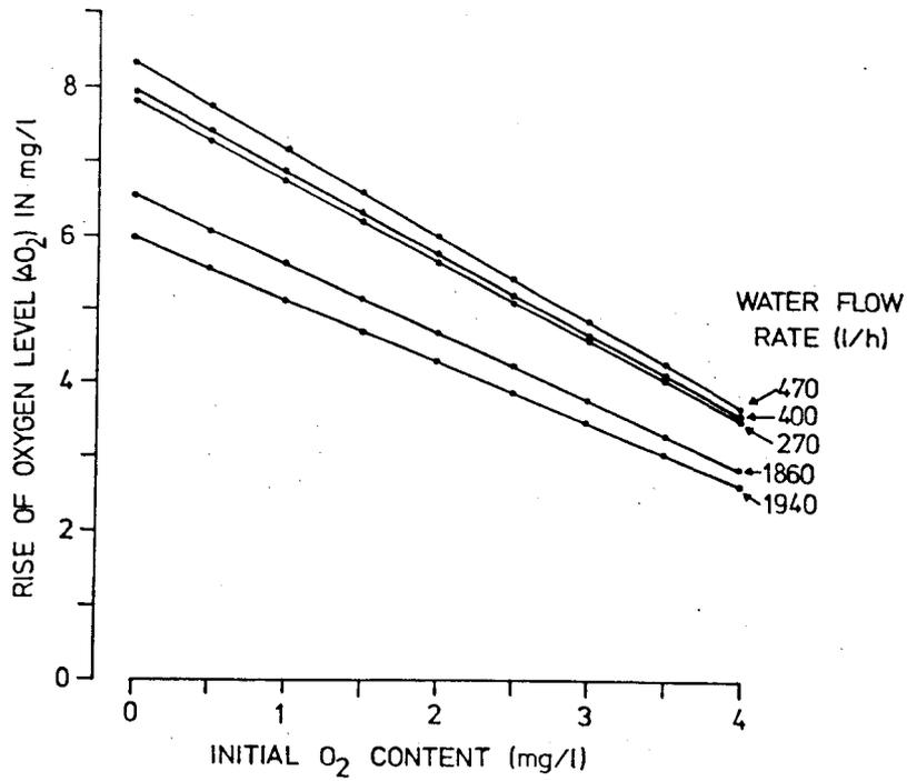
Fig. 3: Oxygen enrichment in relation to water flow rate and initial oxygen content at a constant air supply rate of 80 l/h.
