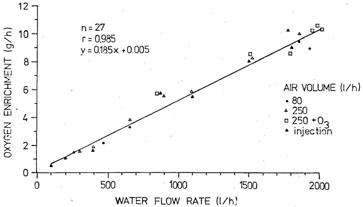
Fig. 6: Oxygen enrichment at different water flow rates and varying air volume introduced.
